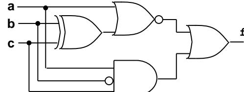
$$f = \bar{a}\bar{b}\bar{c} + \bar{a}bc + a\bar{b}c = \bar{a}(\bar{b}\oplus c) + a\bar{b}c = \overline{a + (b \oplus c)} + a\bar{b}c$$
