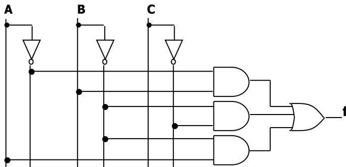
✓  $F(A, B, C) = \prod(M_0, M_3, M_5, M_7) = \sum(m_1, m_2, m_4, m_6) = \bar{A}\bar{B}C + \bar{A}B\bar{C} + A\bar{B}\bar{C} + AB\bar{C} = \bar{A}\bar{B}C + \bar{C}(\bar{A}B + A\bar{B} + AB)$
