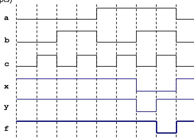
d) Complete the timing diagram of the logic circuit whose VHDL description is shown below: (6 pts)
